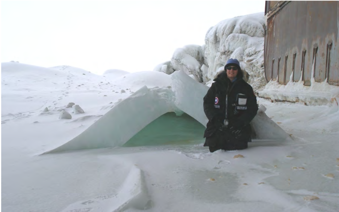
Figure 18: Photograph showing an ice buckle at the SDC drilling platform at the Paktoa C-60 drill site.
