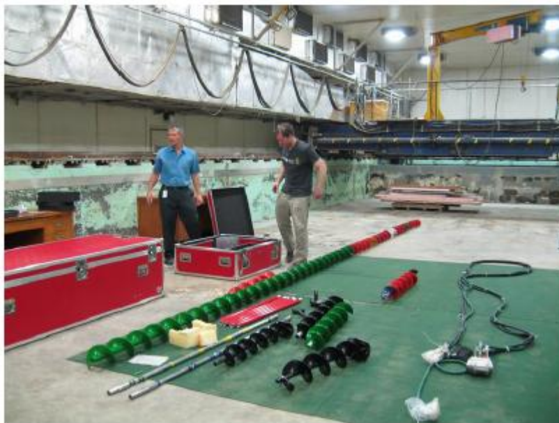
Figure 6. Some of the gear needed for field program. Drill frame is in large red box. The green and red auger shows the depth to which the ice will be drilled (12 m) and tested with the borehole indenter (far right).
