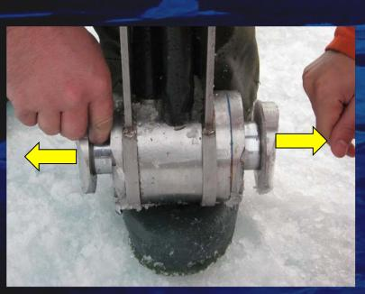
NRC borehole indentor has two faces that each penetrate the ice by 25 mm (1 inch)
