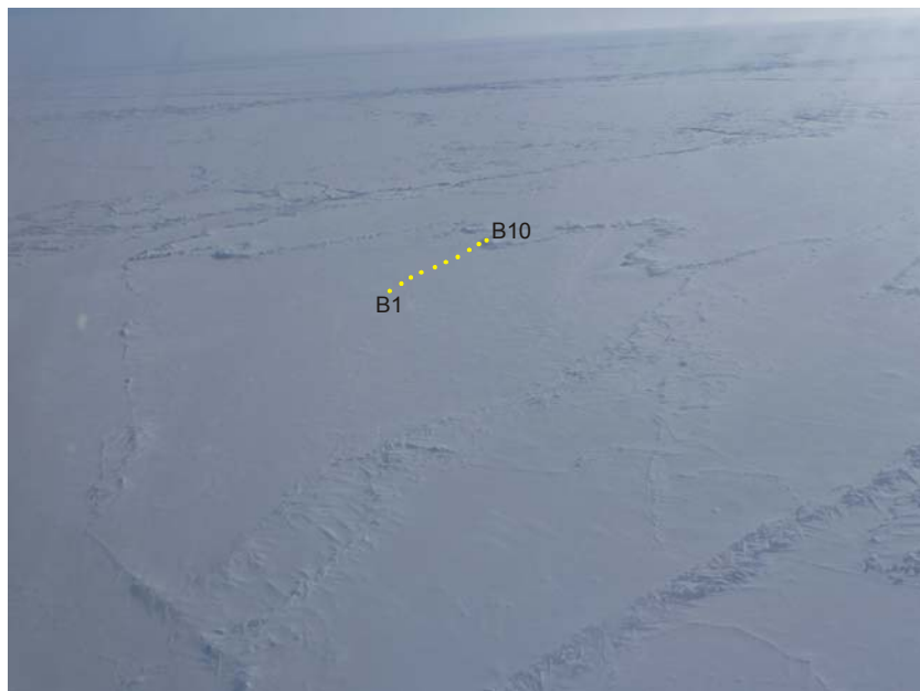
Figure 23 Transect B made on Floe 1 which was likely was first-year ice rather than old ice. What had been identified as old ice in the satellite imagery had drifted further west since the date of the satellite overpass.
