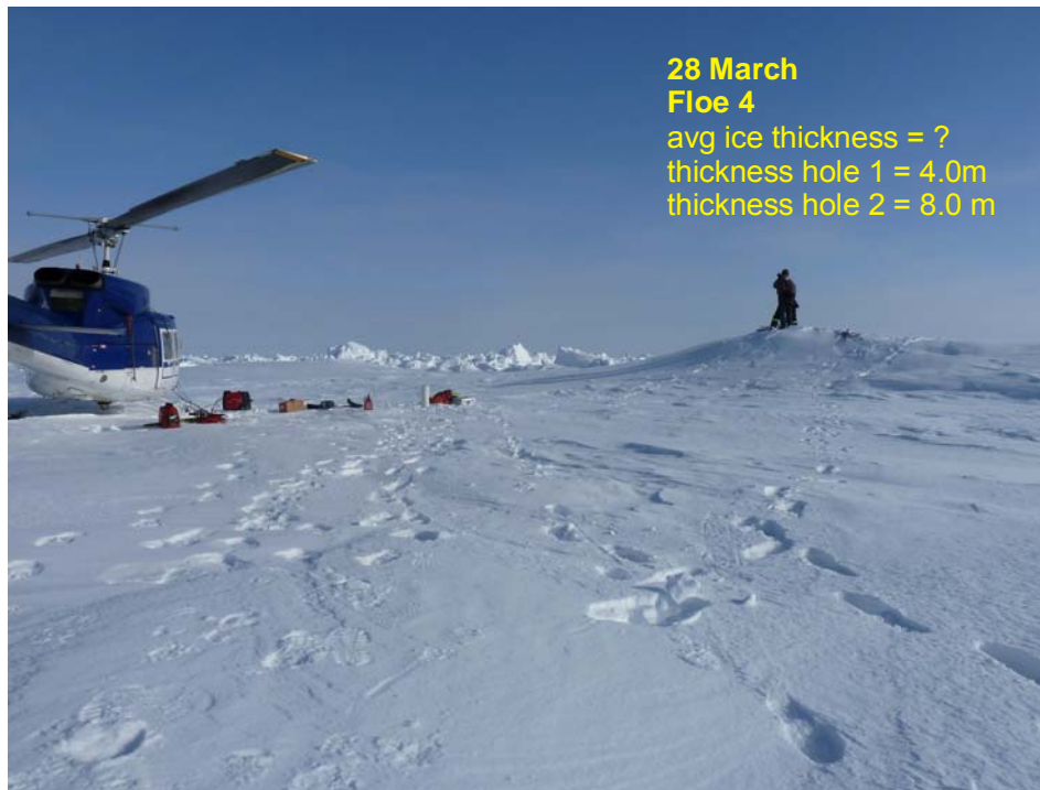
Figure 30 Thicknesses were 4.0 and 8.0 m at two drill holes on Floe 4 (~250 m across).
